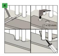
Act similarly in the case of a bigger number heating system pipes. The cut panel elements must be joined with the assembly adhesive for plastic elements.
