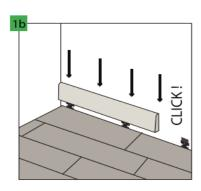
Expansion joints along the walls must be covered with a decorative strip, assembling it by means of glue or special clips. It is recommended to use the Afirmax strips dedicated to a given panel, which guarantee the excellent colour match and the coat resistant to scratching.
