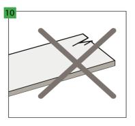
Before and during the installation, control all the panels in the optimal lighting conditions. Do not use defective panels.
