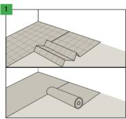
Lay the Arbiton, Ewifoam or Afirmax underlay perpendicularly to the direction in which panels are laid. The neighbouring ribbons of underlay must be fit tightly and joined by means of an overlap or Arbiton AluTape, without leaving any redundant space.
