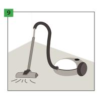
Make sure that the substrate is dry, flat, stable and free of any grease or chemical substances. The protruding irregularities must be scratched off and removed. Before the installation, the ground must be swept and vacuumed carefully so as to remove any contamination. It is necessary to repair any more serious imperfections of the substrate and large cracks.
