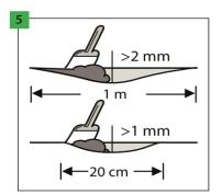
Make sure that the substrate is completely flat. All substrate irregularities exceeding 1 mm, with a length greater than 20 cm, or exceeding 2 mm with a length greater than 1 m must be levelled. Check if the use of the priming or sealing material is necessary. In order to prepare the substrate perfectly, spread the grout or the self-levelling compound on the entire surface.
