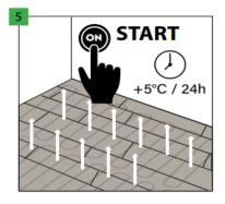
After laying the floor and waiting 24 hours, you can turn on the underfloor heating, remembering to gradually increase the temperature (5°C per day).
