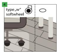
Used office chairs with W-type castors, protecting the floor additionally by means of the protective net. The furniture legs must be provided with protective pads which provide protection against scratching, e.g. made of falt
