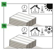
If the temperature is >5 °C during transport, the acclimatization time in a room with a temperature of 18-30 °C should be min. 24 hours. However, in case of temperature ≤5 °C during transport, acclimatization time in a room with a temperature of 18-30  $^{\circ}\text{C}$  should be min. 48 hours.
